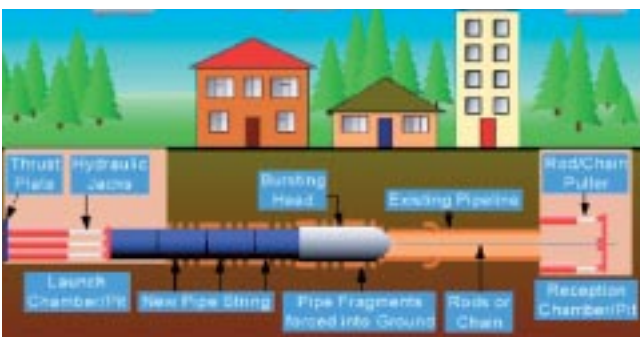
Schematic of pipe bursting
