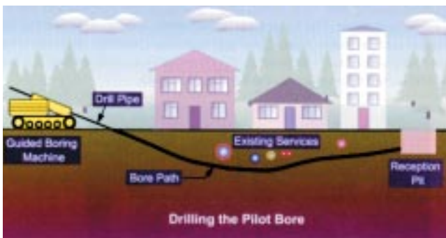
Drilling of the pilot bore (top) and backreaming (bottom) to enlarge the hole and install the pipe.
